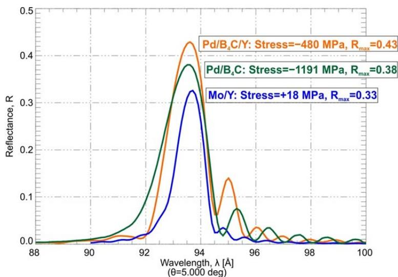
Figure 4. Normal-incidence reflectance of Pd/B<sub>4</sub>C/Y, Pd/B<sub>4</sub>C, and Mo/Y periodic multilayers tuned near 9.4 nm wavelength, as measured using synchrotron radiation at the ALS. The measured stress values for each film are labeled.
