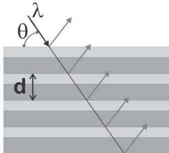
Figure 2. Schematic diagram of a periodic multilayer coating.
