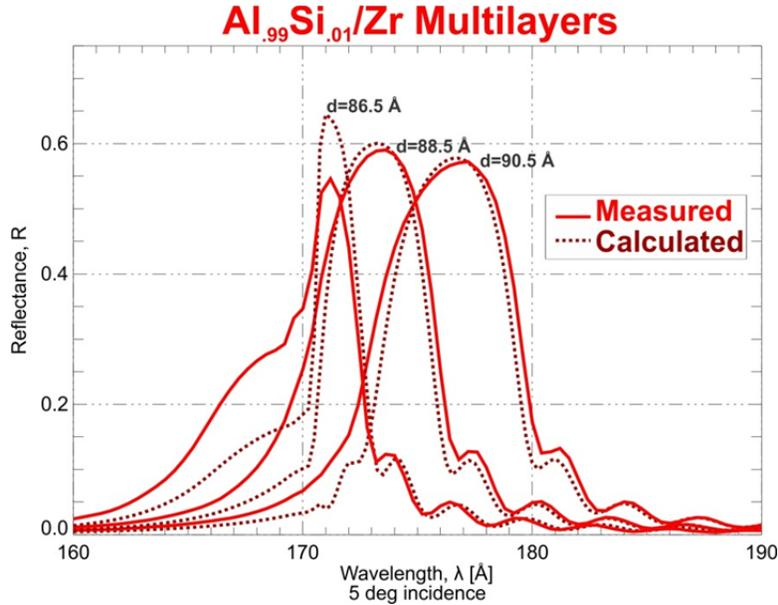
Figure 7. Normal incidence reflectance of periodic Al/Zr multilayers with periods  $d=86.5\text{\AA}$ ,  $88.5\text{\AA}$ , and  $90.5\text{\AA}$ , as indicated. The reflectance was measured at the ALS. Calculations (dotted lines) used optical constants from reference [18], and interface widths  $\sigma=1.35\text{ nm}$ .
