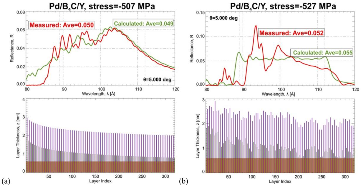
Figure 6. EUV reflectance measured at  $5^\circ$  incidence at the ALS, and modeled using IMD (top), and layer thickness distribution (bottom), for non-periodic multilayers: (a) analytically depth-graded design, and (b) aperiodic design.
