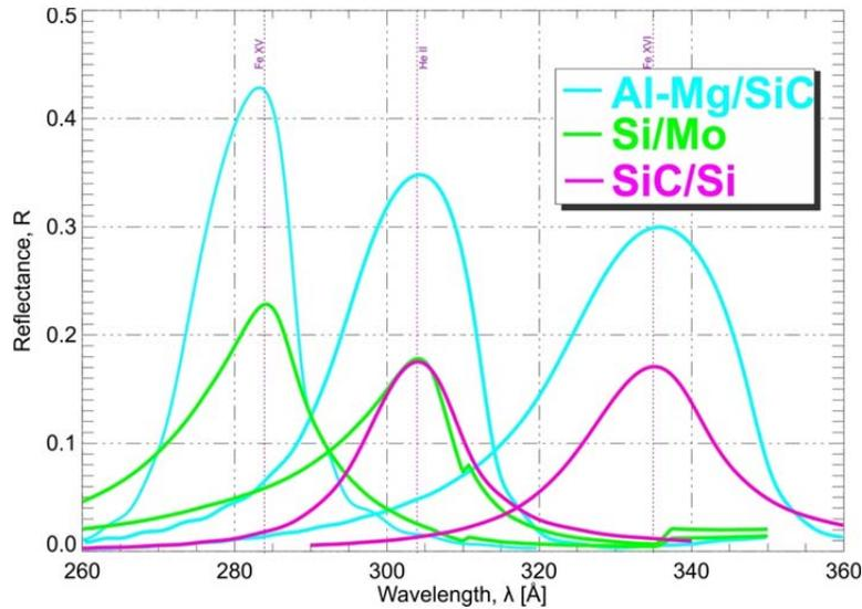
Figure 9. Calculated reflectance curves for periodic Al-Mg/SiC, Si/Mo, and SiC/Si coatings in the 25–35 nm range.
