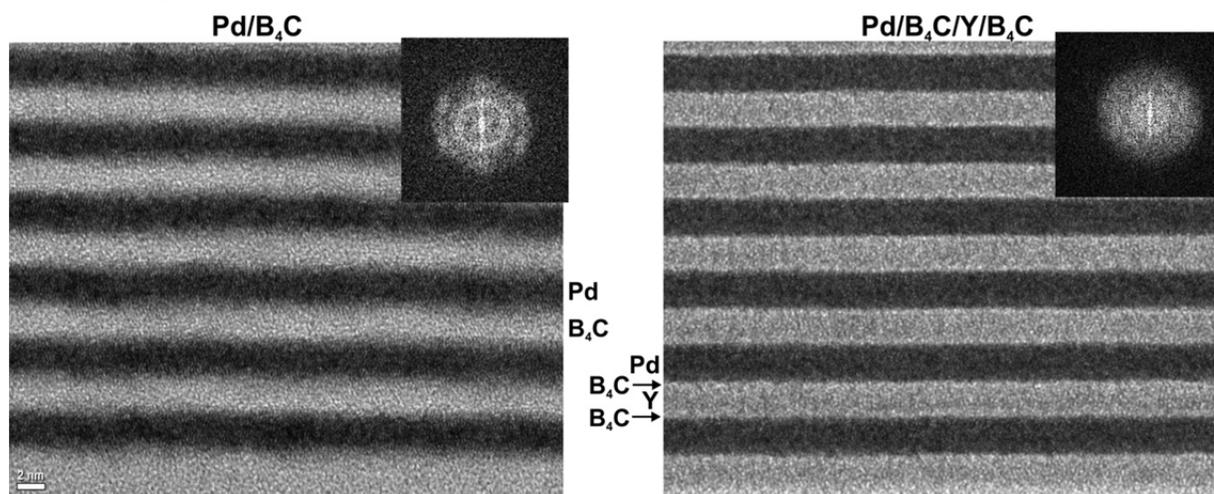
Figure 5. High-resolution transmission-electron-micrographs of multilayers containing repetitions of either Pd/B<sub>4</sub>C (left) or Pd/B<sub>4</sub>C/Y/B<sub>4</sub>C with  $d_{B_4C}=0.6$  nm (right), with a period of  $d \sim 5$  nm in both cases. SAED patterns from each film are shown as insets in the upper right corner in each case.
