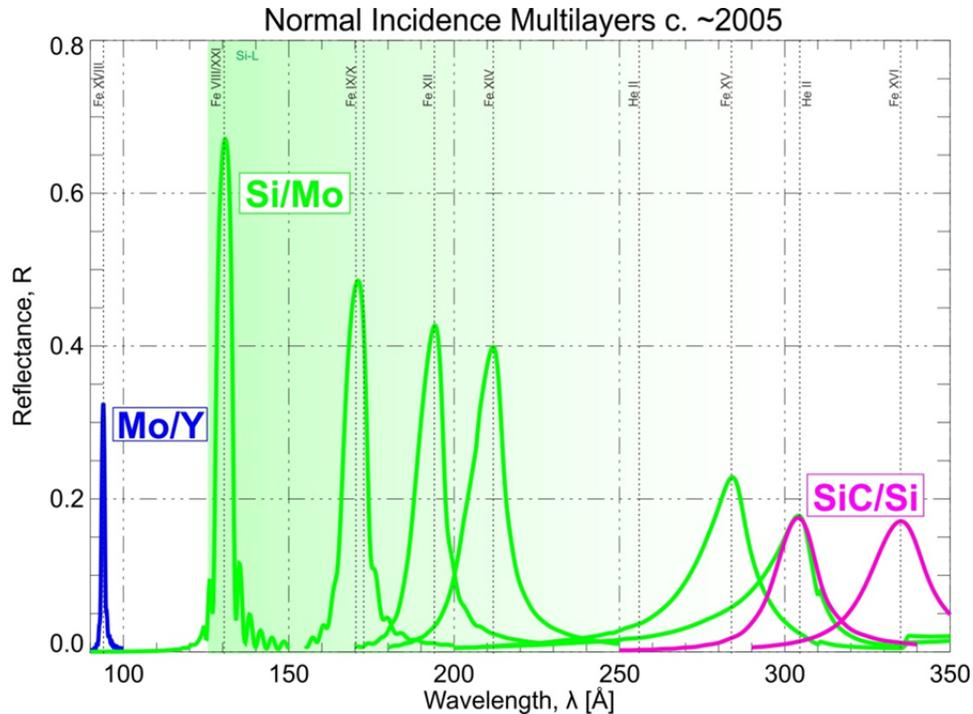
Figure 3. Some of the best normal incidence periodic multilayers that were available for use in solar instrumentation approximately ten years ago.
