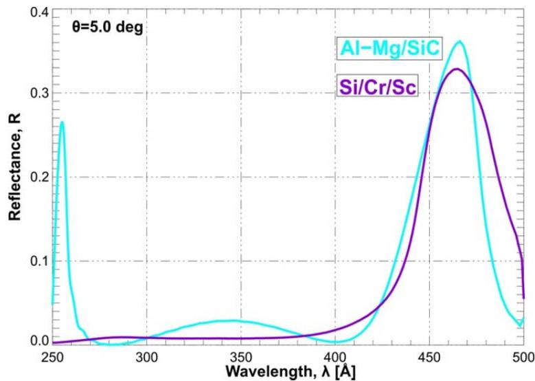
Figure 11. Measured normal incidence reflectance of periodic Al-Mg/SiC and Si/Cr/Sc multilayers tuned near 46.5 nm. The high reflectance in 2<sup>nd</sup> order of the Al-Mg/SiC coating precluded its use in the MOSES instrument.
