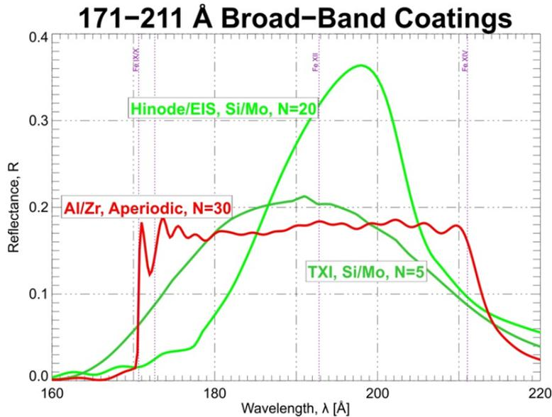
Figure 8. Calculated reflectance of an aperiodic Al/Zr multilayer designed for flat response from ~17 to 21 nm. Also shown are calculated reflectance curves for the periodic Si/Mo coatings used on the Hinode/EIS and TXI instruments.
