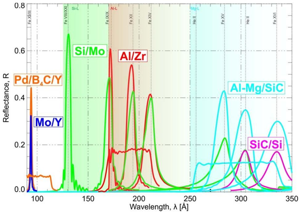
Figure 12. Summary of normal incidence reflectance of current EUV multilayers in the 9 – 35 nm range.
