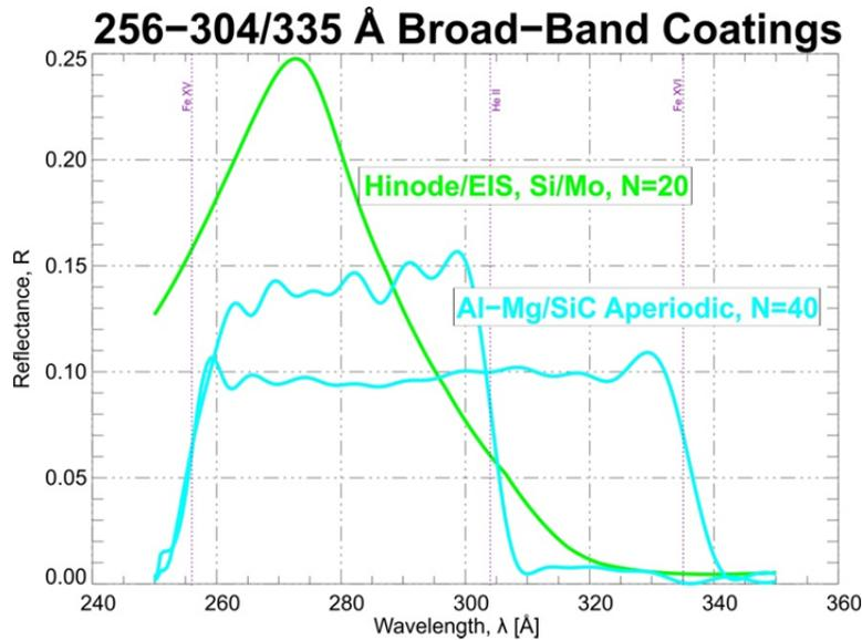
Figure 10. Calculated reflectance of a two aperiodic Al-Mg/SiC coatings designed for flat response from  $\lambda=25$  to 31 nm, and from  $\lambda=25$  to 34 nm. Also shown is the calculated reflectance of the periodic Si/Mo multilayer used for the long-wavelength band on the Hinode/EIS instrument.
