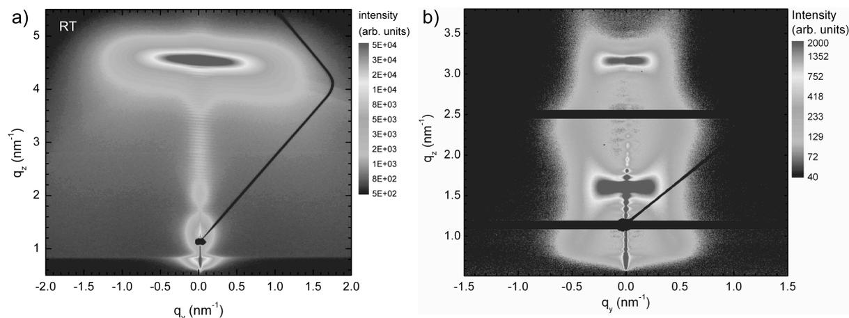
Fig. 1 – GISAXS patterns of (a) W/B<sub>4</sub>C and (b) La/B<sub>4</sub>C multilayer mirrors.
